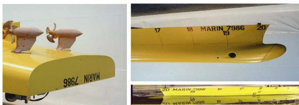
AZIPOD Propulsors and Bow Bulb on Tank Test Model
